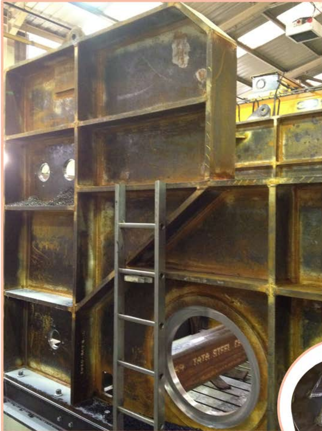
FREE ISSUED FABRICATED STORAGE TANK BEING MACHINED ON ONE OF OUR LARGE CNC MILLING MACHINES.
